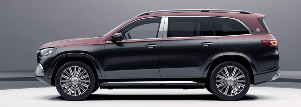
55.9 cm (22-inch) Maybach multi-spoke light-alloy wheels, painted in high-gloss black with a high-sheen finish, including fully integrated wheel bolt covers.
