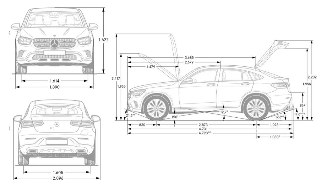
All dimensions in millimetres. The dimensions shown are mean values and apply to standard-specification, unladen vehicles.
