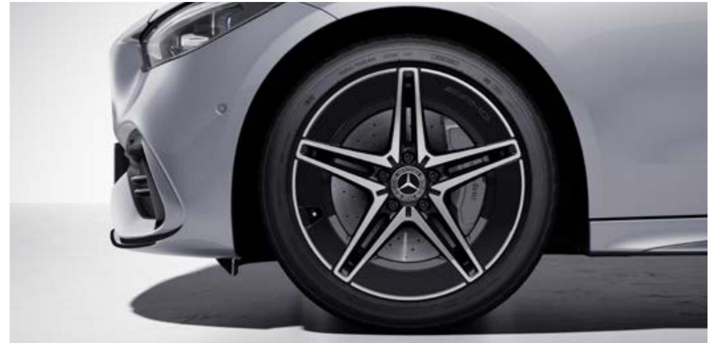
45.7 cm (18 inch) AMG 5-spoke light-alloy wheels aerodynamically optimised, painted black with high-shine finish (Available with C 300d)
