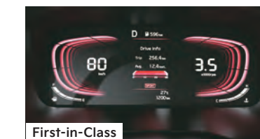
31.7 cm (12.5") Full Segment LCD Cluster with Advanced 10.6 cm (4.2") Color TFT MID
