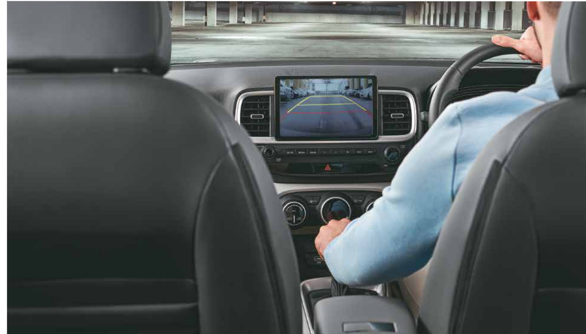
Rear parking assist camera with dynamic guidelines
