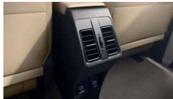
Rear AC Vent with Charging Ports
