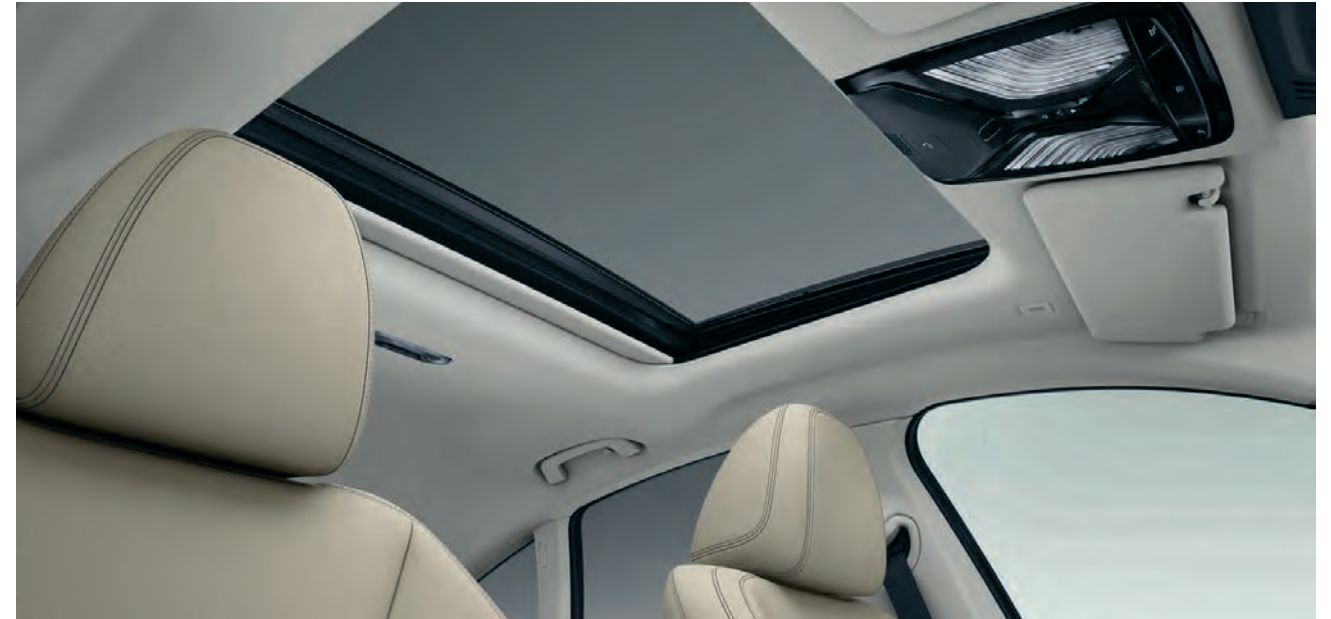
■ The glass sunroof with slide and lift function, including an electric sliding interior roof, anti-trap protection, as well as comfort opening and closing, allows the airflow to be individually regulated to create a pleasant interior climate. The integrated wind deflector prevents draughts from developing in the interior and ensures a lower level of wind noise.
