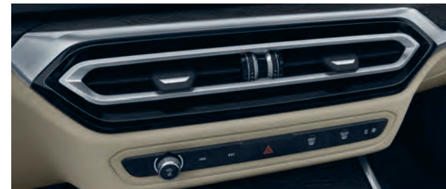
■ The Automatic air conditioning with 3-zone control and automatic temperature control features separate controls for you and your front passenger, as well as for the passengers in the rear. It also includes Automatic Air Recirculation (AAR), a micro active carbon filter, a fog and solar sensor, as well as rear air vents with a digital display.
