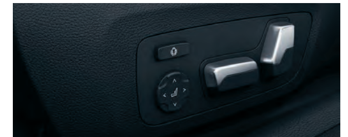
■ The electric seat adjustment makes it particularly convenient and easy to adjust the driver and front passenger seats. The memory function enables drivers to save and retrieve their desired settings for the driver's seat and exterior mirrors at the push of a button.
