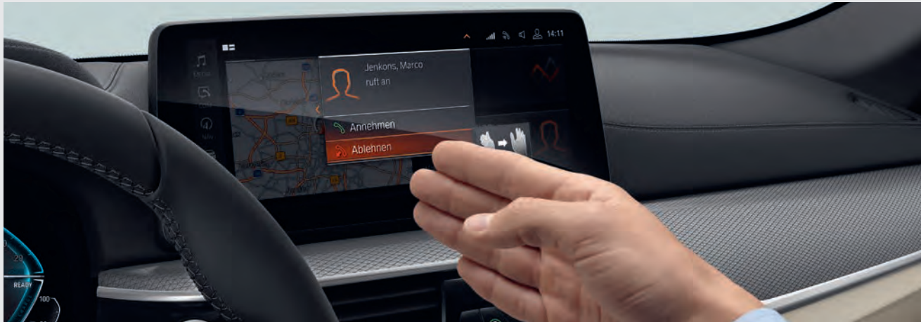
With BMW Gesture Control , selected functions can be operated by means of defined hand movements. Simple gestures such as 'swiping' or 'pointing' are identified in the recognition area above the centre console and trigger functions such as accepting or rejecting an incoming telephone call, proceeding or cancelling navigation as well as starting and ending voice recordings.
