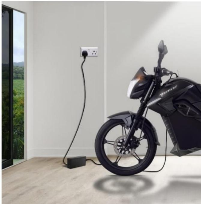
The charger provided with the Li-Ion battery is sophisticated and is a special purpose electronic charger. This charger has an additional safety feature which provides protection from output overvoltage, output overcurrent and short-circuit. The charger is designed to charge only eTryst 350<sup>®</sup>.
