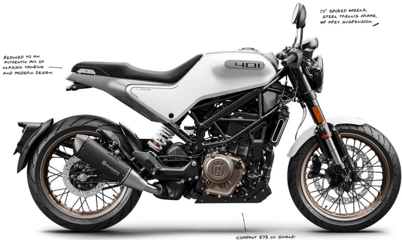
COMPACT 373 CC SINGLE-CYLINDER ENGINE DELIVERING AN IMPRESSIVE 44 HP AND 37 NM OF TORQUE.
