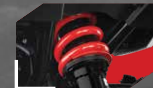
PRE-LOAD ADJUSTABLE REAR SUSPENSION 220 MM LONG TRAVEL
